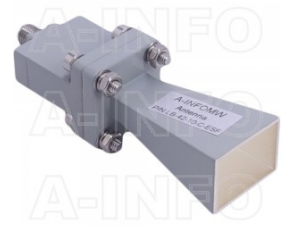
LB-42-10-C-ESF Standard Gain Horn Antenna 18-26.5GHz 10dB Gain Endlaunch SMA Female
